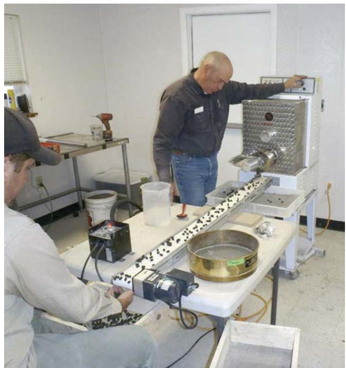
Figure 2. Production of extruded seed pellets with a TR-100 Pasta Machine. Photo by Matthew Madsen
