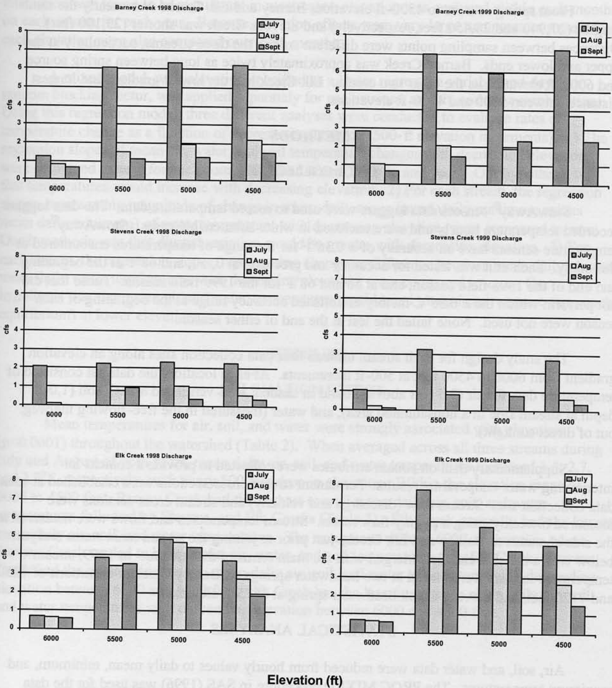
Figure 2. Stream flow discharges for Barney, Stevens, and Elk Creeks, at 6000, 5500, 5000, 4500-ft elevations, for beginning July, August, and September, 1998 and 1999.
