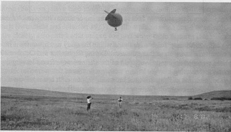
Figure 5. Using helium blimp for aerial photography.
